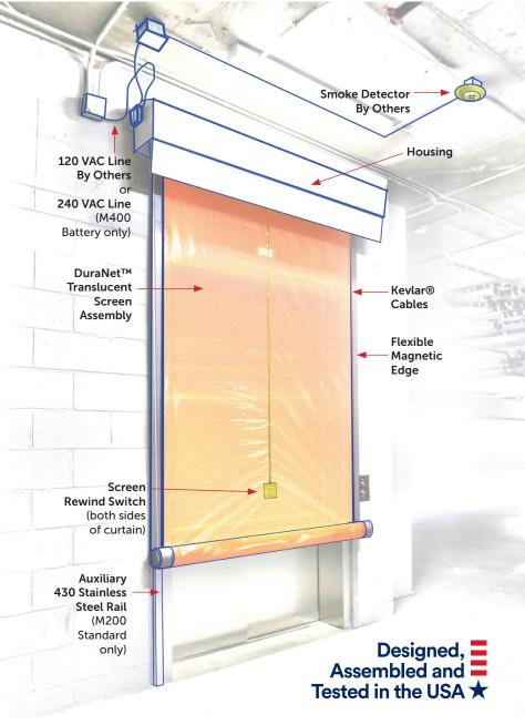
Rewind Switch. The Smoke Guard system screen rewind switch may be activated from both sides of the screen. This feature allows elevator occupants to exit from the elevator car using the interior (shaft side) of the switch. The screen will then redeploy after egress, as long as the smoke detector continues to be activated. In the event of power outage, the vertical edge of the curtain can be pushed away from the rail to allow passage with a force less than 15 lbs. as required by the IBC.
